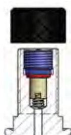
Model of valve stem integrated 7/8"14 UNF (C)
