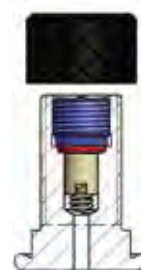
Model of valve stem integrated 7/8" 14 UNF (C)
