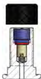
Model of valve stem integrated 7/8"14 UNF (C)
